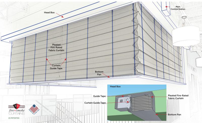
**System Operation.** The system is deployed upon a signal from the local smoke detection system or a smoke control panel. System requires 120-240 volt power. The unit is also equipped with a 24 volt DC battery back-up system that maintains the electronic controls. When required the system can be connected to building standby power. The controls include a universal power supply that supports either 120 or 240 volt operation.
