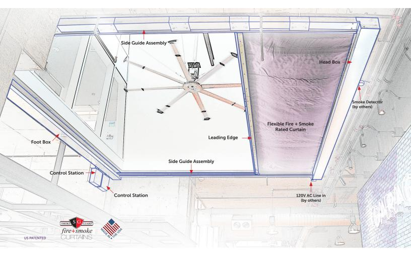
**System Operation.** The system is deployed upon a signal from the local smoke detection system or a smoke control panel. System requires 120 or 240 volt AC. The unit is also equipped with a 24 volt DC battery back-up system that maintains the electronic controls. When required the system can be connected to building standby power. The controls include a universal power supply that supports either 230 or 240 volt operation.
